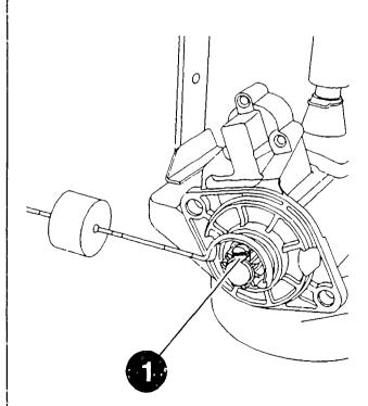
Checking clutch overrunning torque
